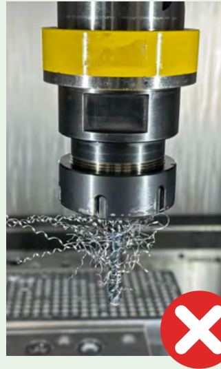
Competitor C tool after 16 threads
