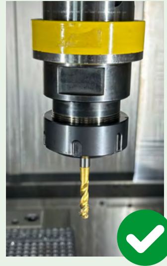
LITELINE tool after 25 threads
